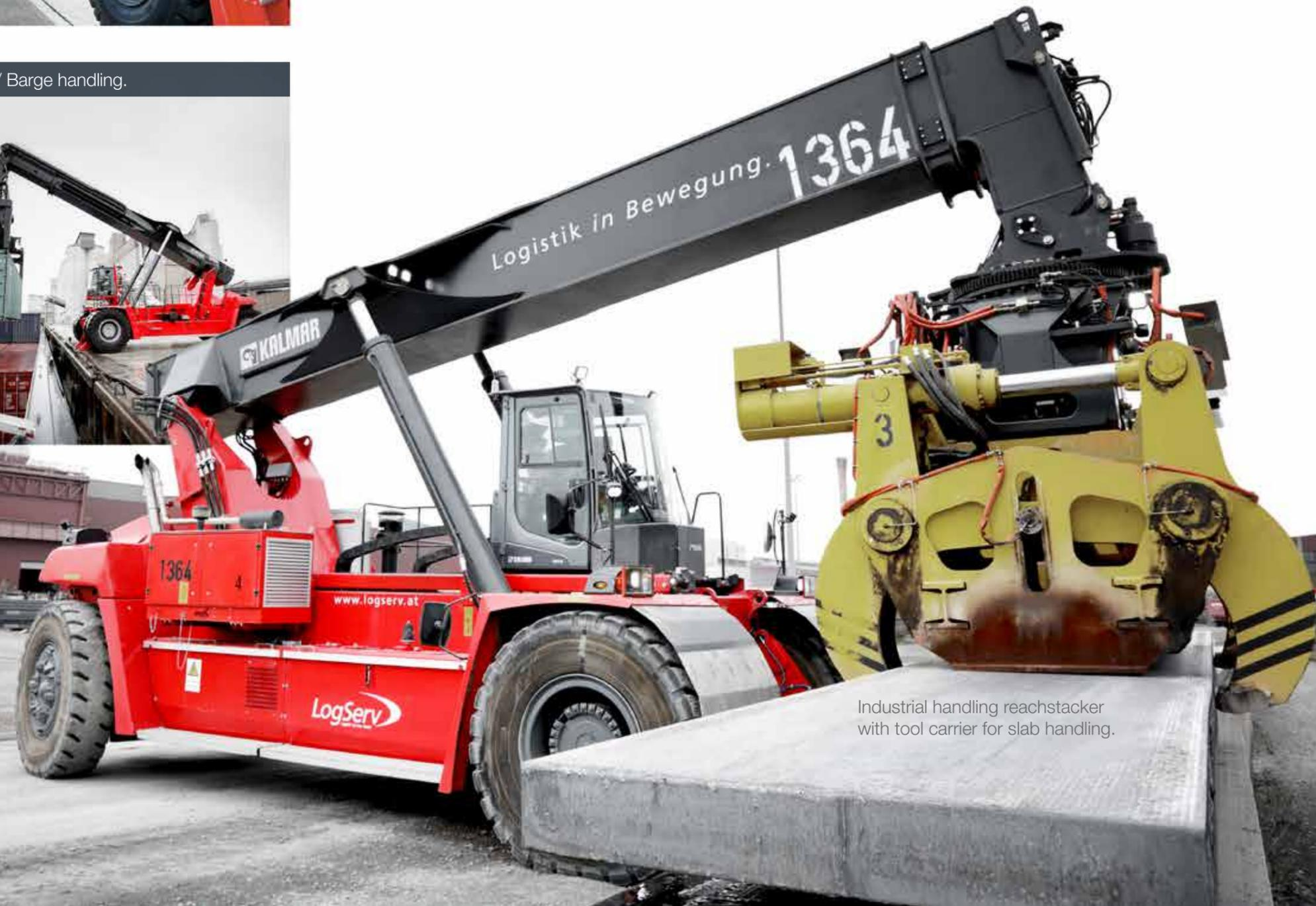
Industrial handling reachstacker with tool carrier for slab handling.
