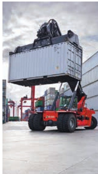
Containerumschlag - Top-Lift (S)
