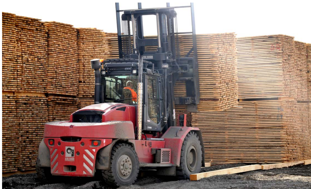
Designed specifically for the lumber industry: A reversible cooling fan helps clear the cooler from harmful dust. The rotatable driver's seat lets the driver go 'forward in reverse' with unobstructed view even when fully loaded.
